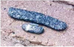
**Lead wheel weights with damage from traffic. The bits of worn lead can wash into our waterways.**
